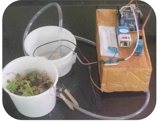
Moisture Detection Automatic Watering System
