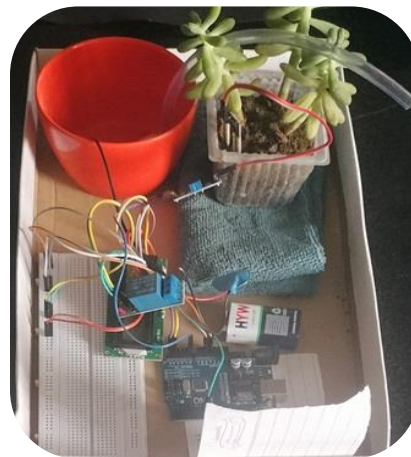
Automatic Plant Watering System
