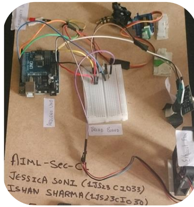
Hazardous Gas Detection and Alarming System
