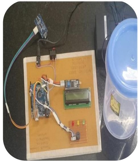
Arduino based Water level Controller
